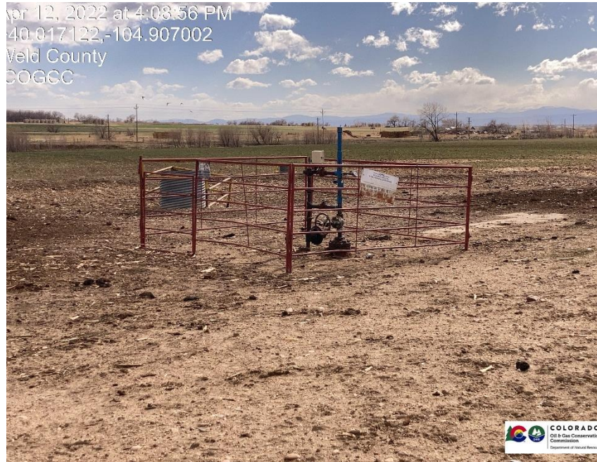
Pic 1 wellhead, plunger lift.
