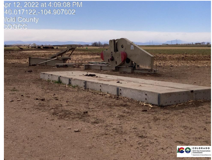
Pic 2 pump jack equipment on location needs to be removed.
