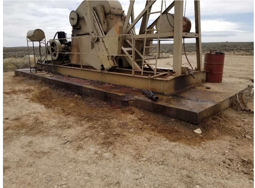
Photo 4. Spill at pump jack.
