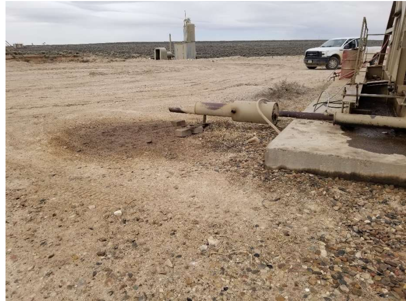
Photo 8. Stained soil at pump jack exhaust.
