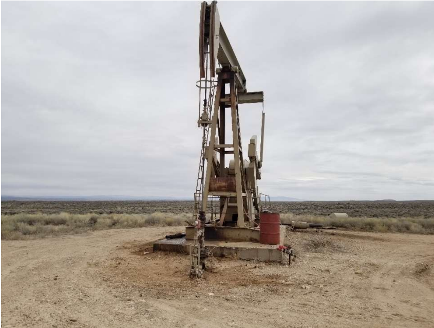
Photo 3. Stained soil at wellhead. Chemical container with no secondary containment.
