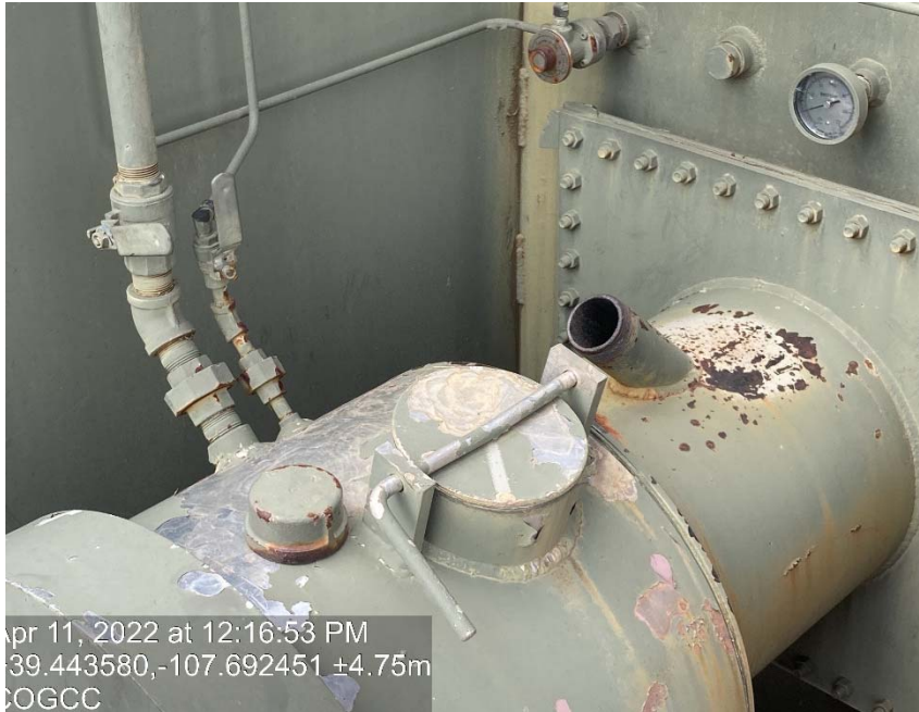
Cap on burner not installed and burner is running
