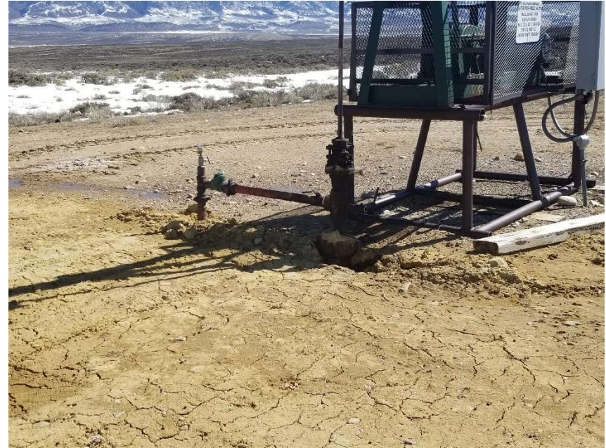
Photo 2. No bradenhead access apparent.
