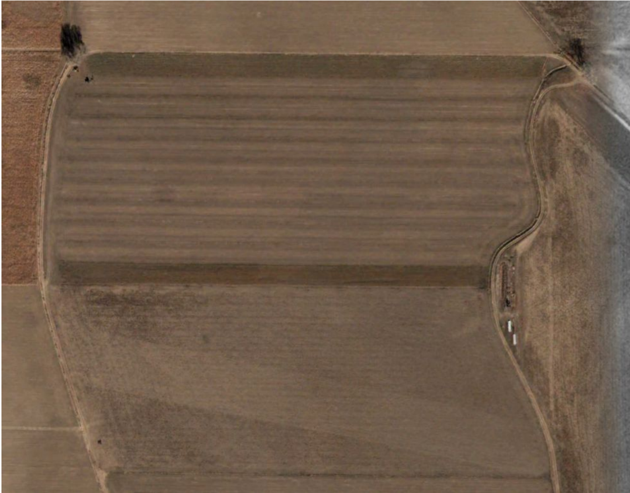
Photo 1. Google Earth aerial imagery taken 12/11/2002 prior to the development of the Groves #43-34 location. Photo illustrates there is not a pre-existing road prior to the development of the location.
