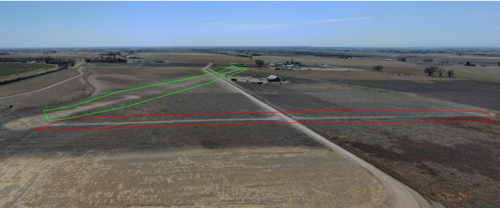
Photo 8. Drone aerial imagery illustrates the access road that has not been reclaimed (red) and the flowline area (green).
