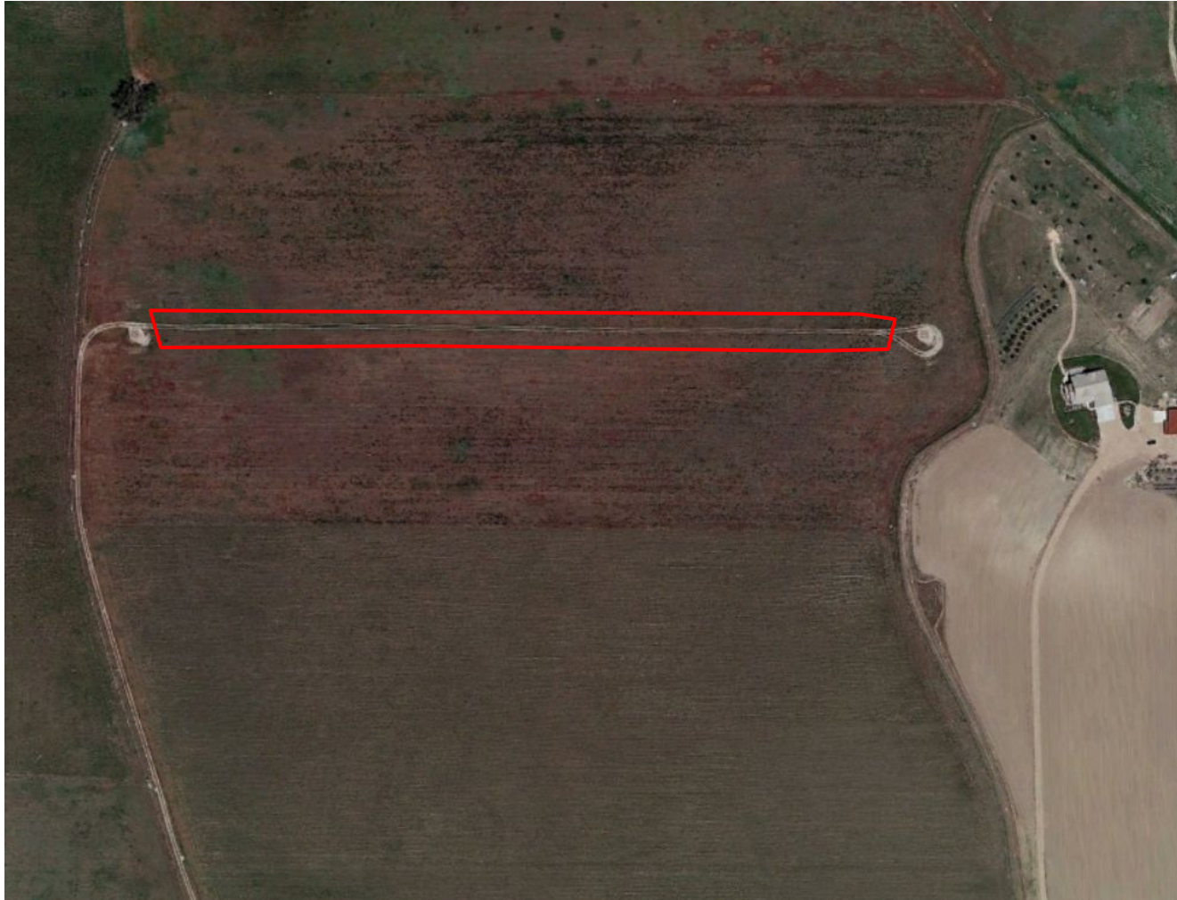
Photo 2. Google Earth aerial imagery taken 6/19/2014 during active operations of the Groves #43-34 location. Photo illustrates an access road was in use for the location. This access road remains and has not been reclaimed per Rule 1004.
