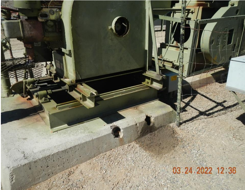
Concrete pad is wet and stained beneath prime mover. Soil adjacent to prime mover is stained.
