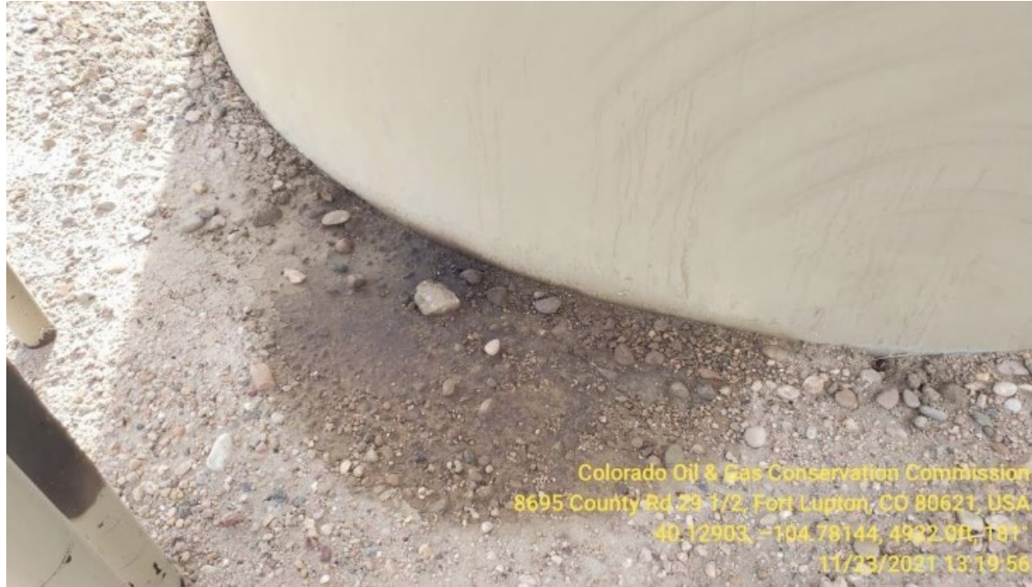
Photo 11 – Oily soil on east side of crude tank documented in Inspection #699304532 on 11/23/21
