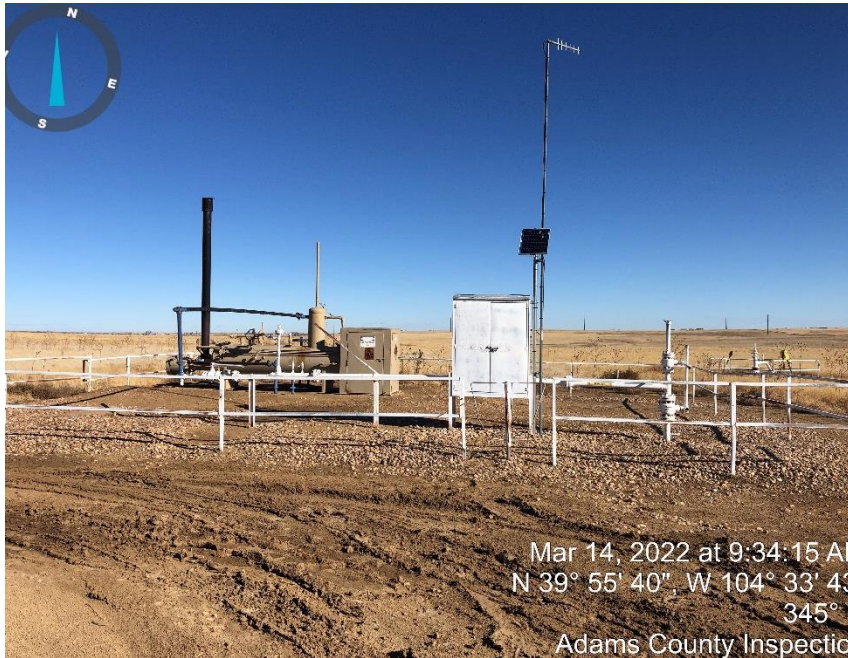
Photo #3 Separator, meter, RTU.
