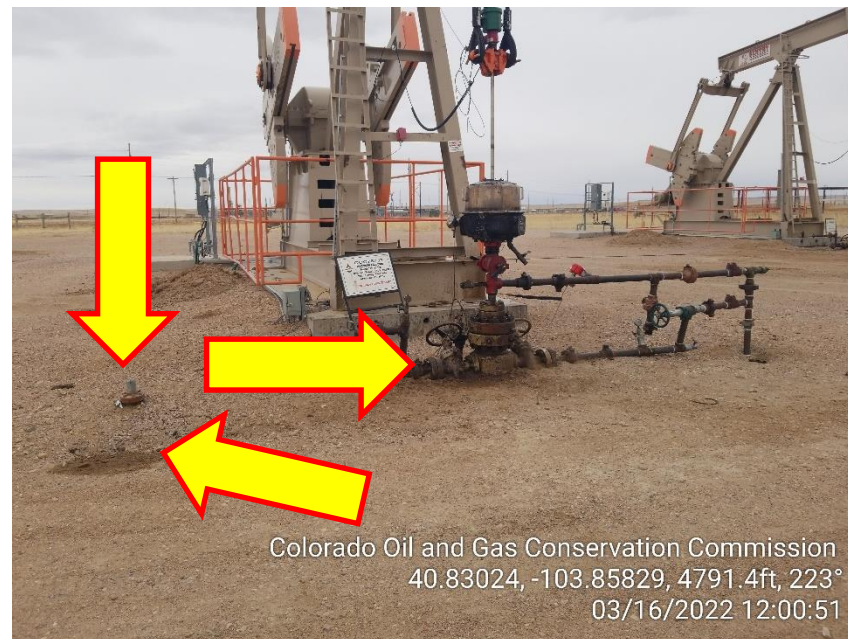
Photo 6 – 2207 Wellhead – Unmarked Riser and Stained Soil
