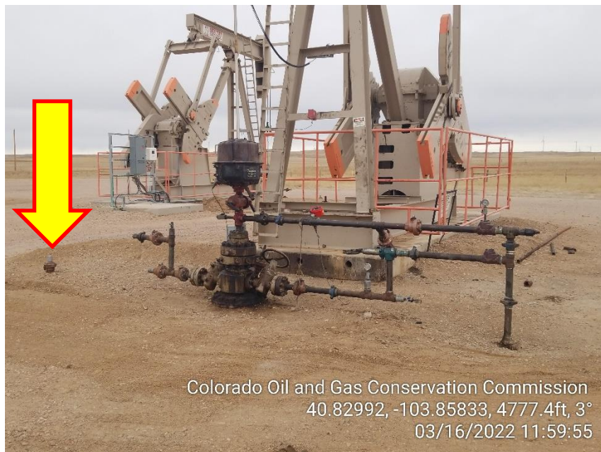
Photo 3 – 2208B Wellhead – Unmarked Riser
