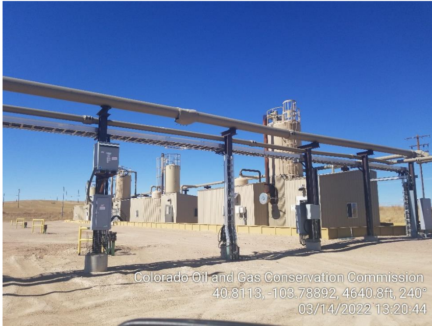
Photo 21 – Heater Treaters
