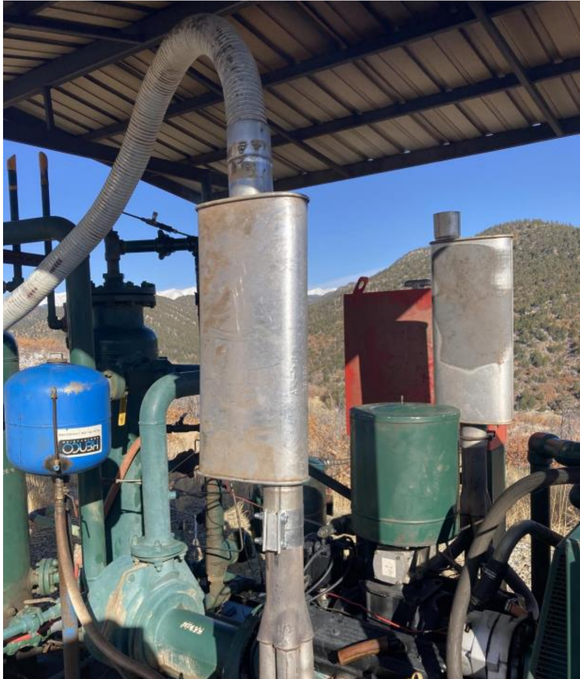
PHOTO 2: THE MUFFLER ON THE COMPRESSOR SKID HAS BEEN REPLACED AND ALL ENGINE COMPONENTS HAVE BEEN CHECKED TO ENSURE GOOD MECHANICAL CONDITON.
