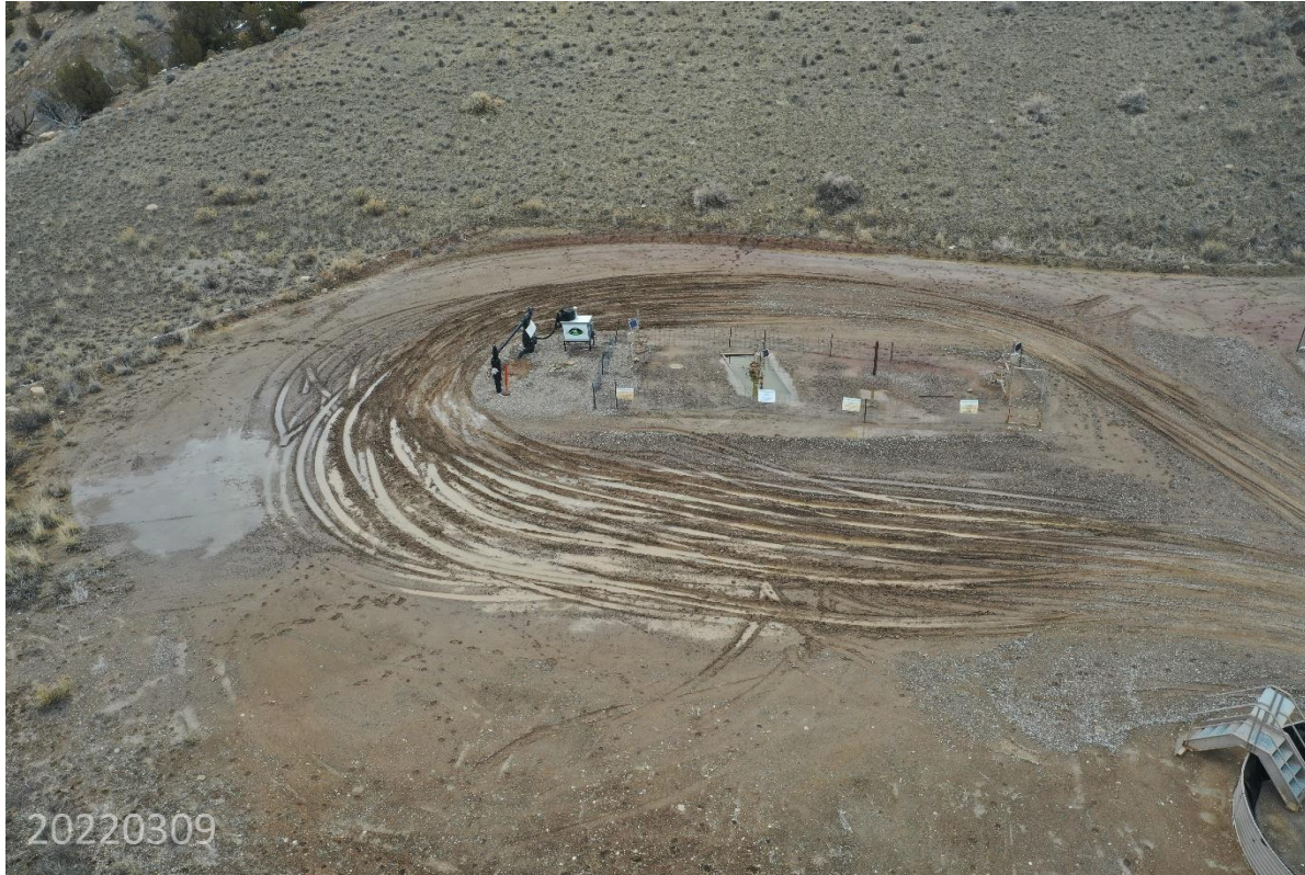
Photo 1: Photo taken with use of a sUAS. Photo taken from southwest end of the Location, facing northeast. Photo provides an overview of the Location showing control measures to stabilize the working pad, minimize rutting, tracking and sediment transport remains missing or insufficient.
