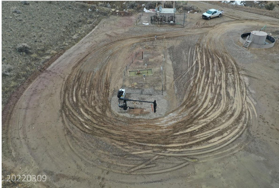
Photo 2: Photo taken with use of a sUAS. Photo taken from northwest end of the Location, facing southeast. Photo provides an overview of the Location showing control measures to stabilize the working pad, minimize rutting, tracking and sediment transport remains missing or insufficient.
