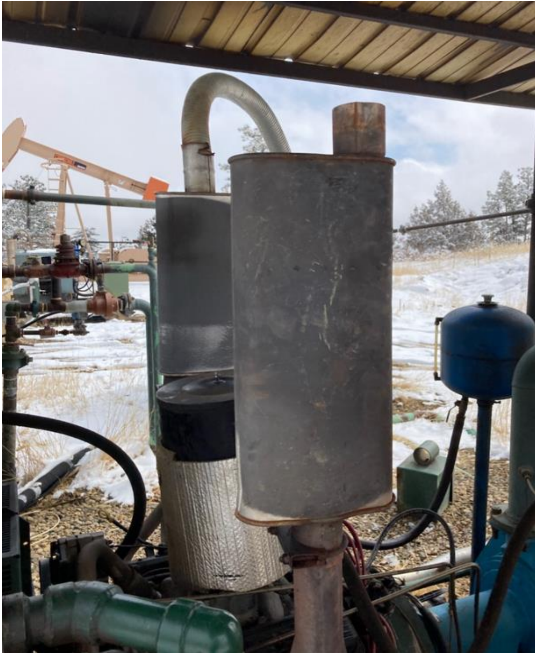
PHOTO 1: MAINTENANCE TO THE ENGINE HAS BEEN PERFORMED AND THE MUFFLER REPLACED TO ENSURE GOOD MECHANICAL CONDITION. THE SELF INSPECTION PROCESS HAS BEEN REVIEWED.
