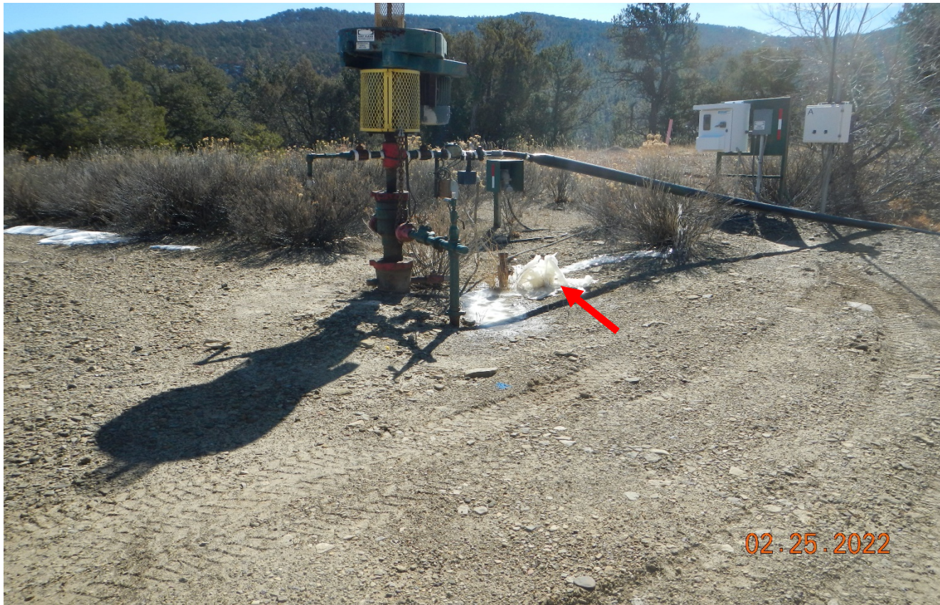
Photo 2. There appears to be a water leak near the wellhead.
