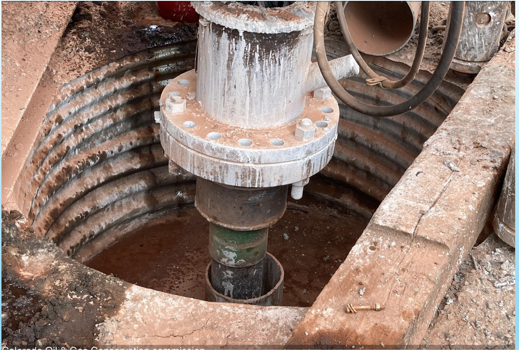
PHOTO 3: DIVERTER INSTALLED WITHOUT BOP.
