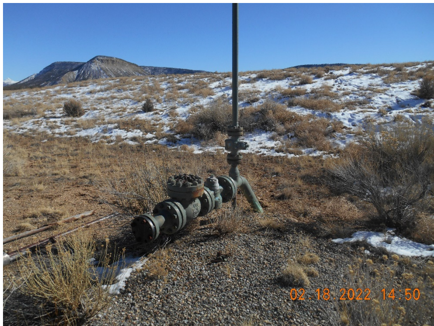
Flowline riser locked out/tagged out
