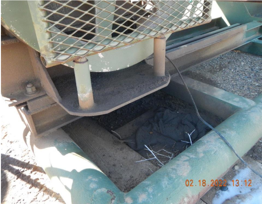
Stained ground around pump jack.
