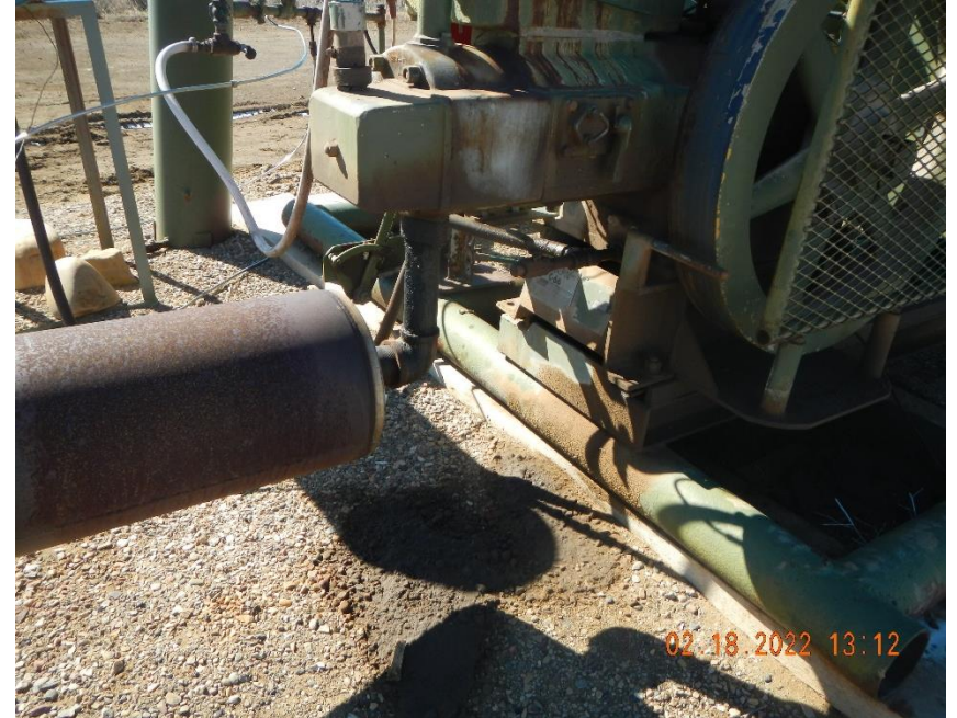
Stained ground around pump jack.
