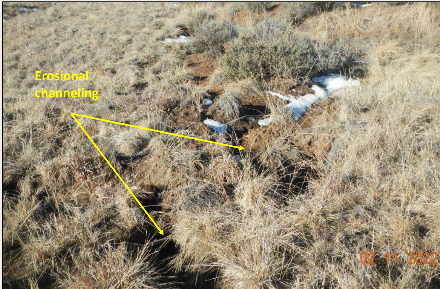
Photo 4. Erosional channel approx. 1ft wide and 2.5ft deep observed in the western project area, deepening as it flows toward the edge of the project area. Stabilization measures are needed here.
