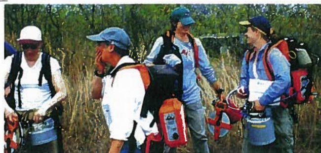
a group of researchers during a flux mapping fieldwork, using the WS-L1820 flux meter Courtesy of United States Geological Survey
