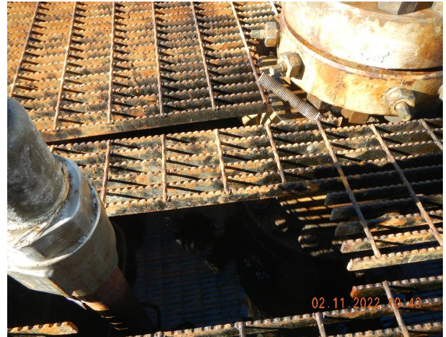
Hydrocarbon fluid in cellar.
