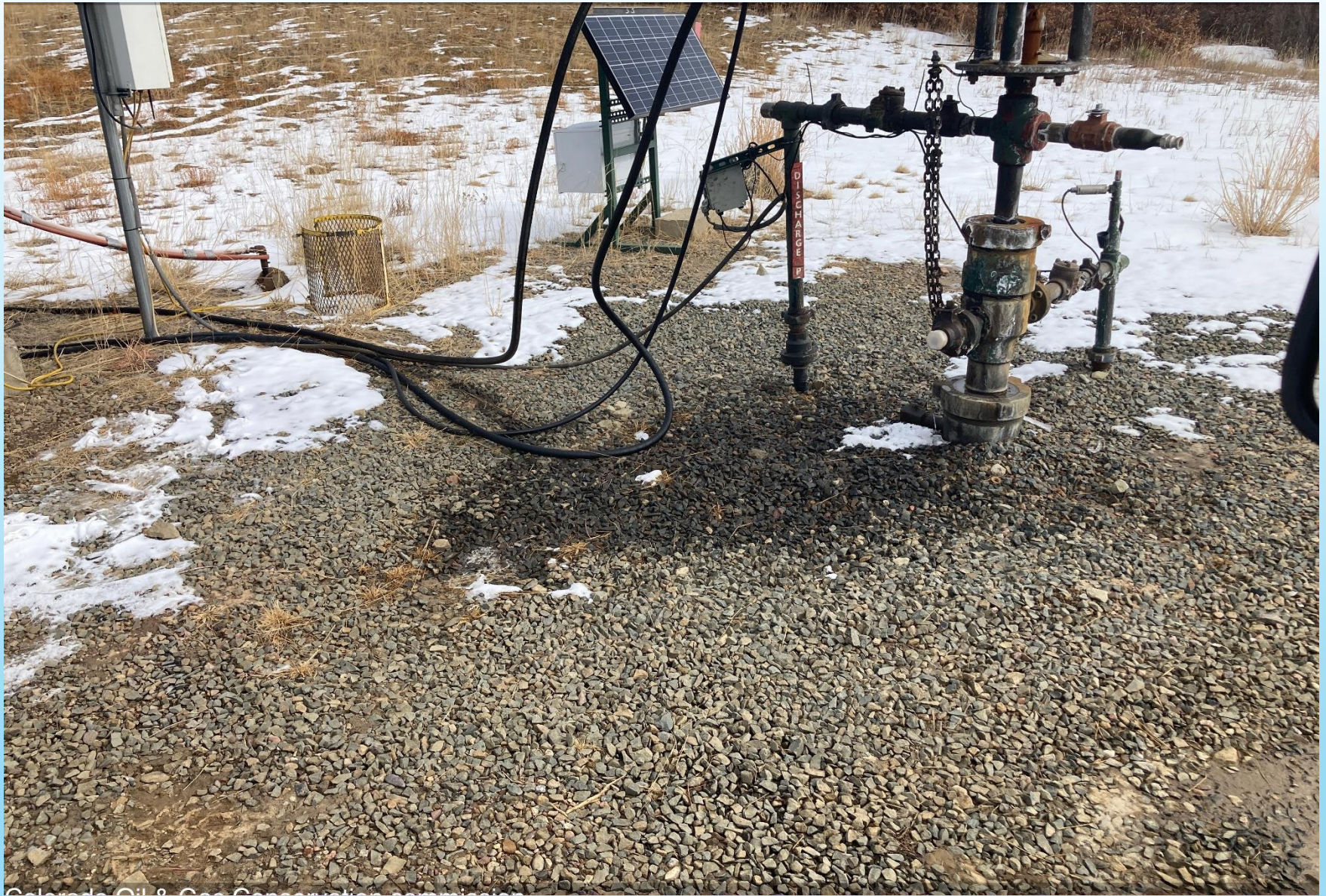
PHOTO 3: AREA OF IMPACTED SOIL AROUND WELLHEAD (APPEARS TO BE HYDRAULIC OIL FROM LEAKING HOSES). Conduct maintenance on equipment, cleanup stained material and review self inspection processes. COMPLY WITH RULE 1002,,(2).D. CA DATE 02-03-2022. THIS IS THE SECOND NOTICE IN THE LAST 14 MONTHS OF THIS SAME CONDITION.
