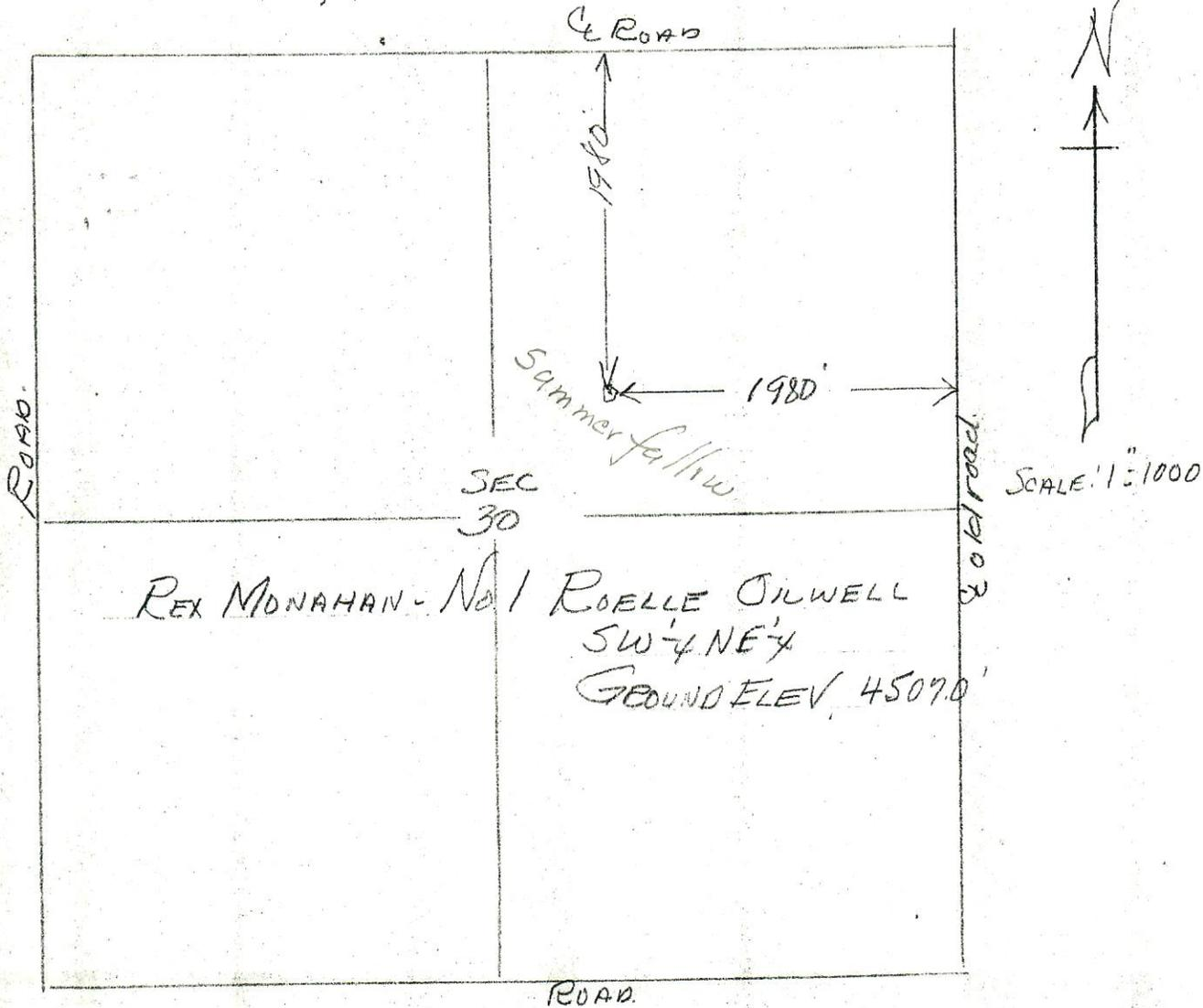
I hereby certify that the above plat is an accurate representation of a correct survey showing the location of Rex Monahan-No.1 Roelle Oilwell in SW 1/4 NE 1/4 Sec. 30 T12N R52W 6PM. The elevation of the ground at the stake is 4507.0 feet above sea level from U.S.G.S. Bench Mark.
