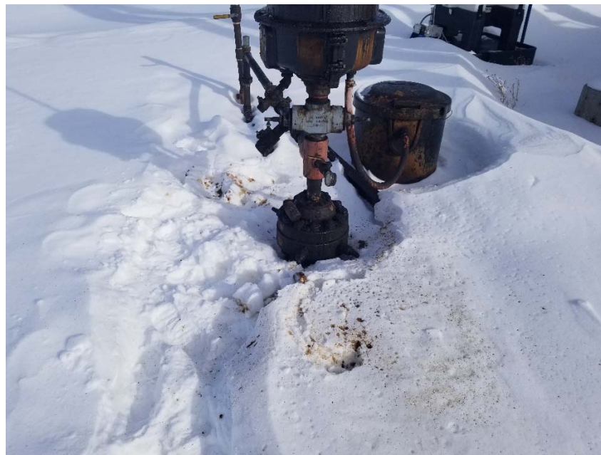
Photo 3. Fresh oil in snow at wellhead.
