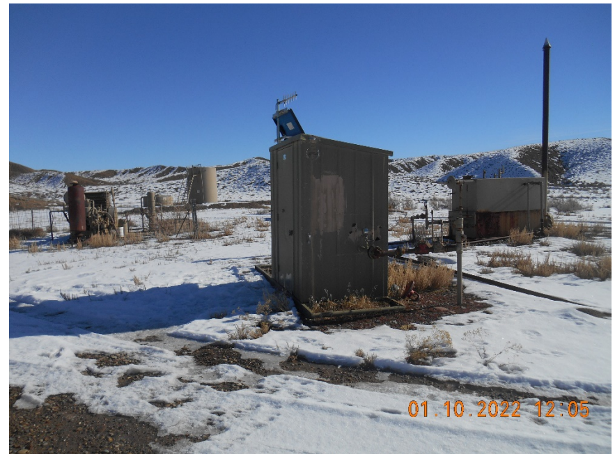
Separator and meter housing
