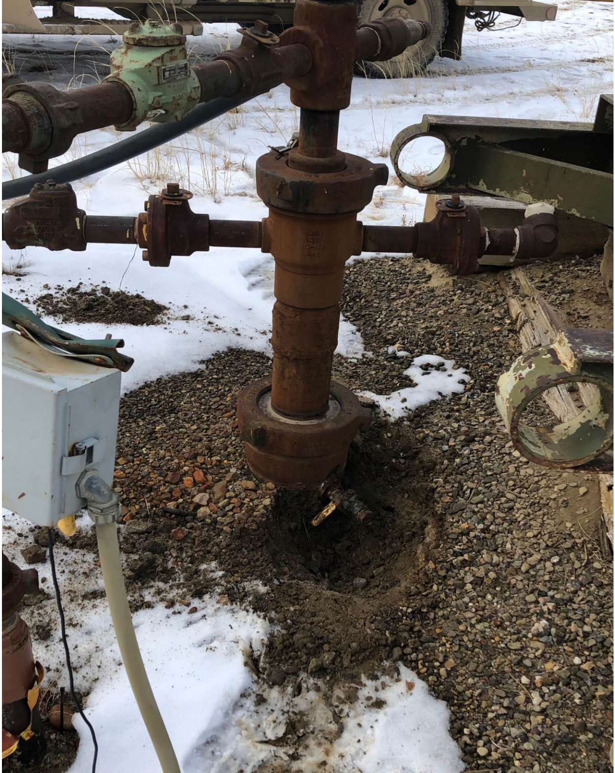
Installed appropriate fittings to allow bradenhead visual inspection as per Rule 419.a.(1), (2).
