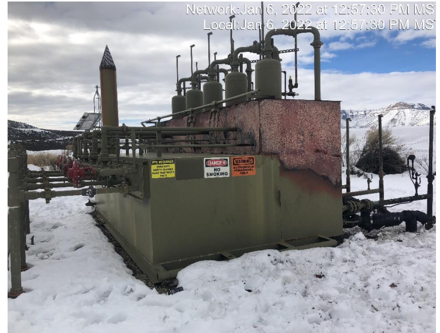
Photo #5607 Separator after fire.
