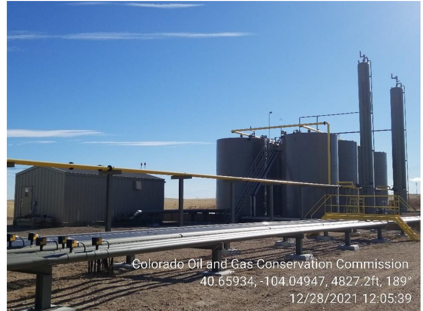
Photo 4 – Tank Battery and LACT
