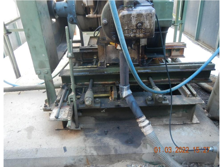
Concrete beneath prime mover is wet and stained.
