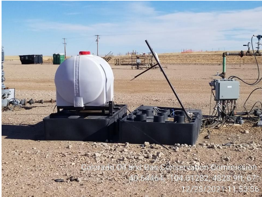
Photo 5 – Chemical Tank missing Label
