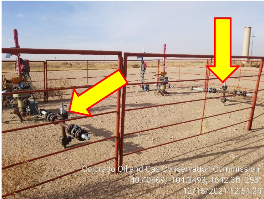
Photo 3 – Unmarked Riser at Wellheads
