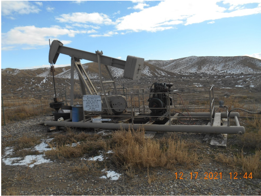
Wellhead with pumpjack and sign
