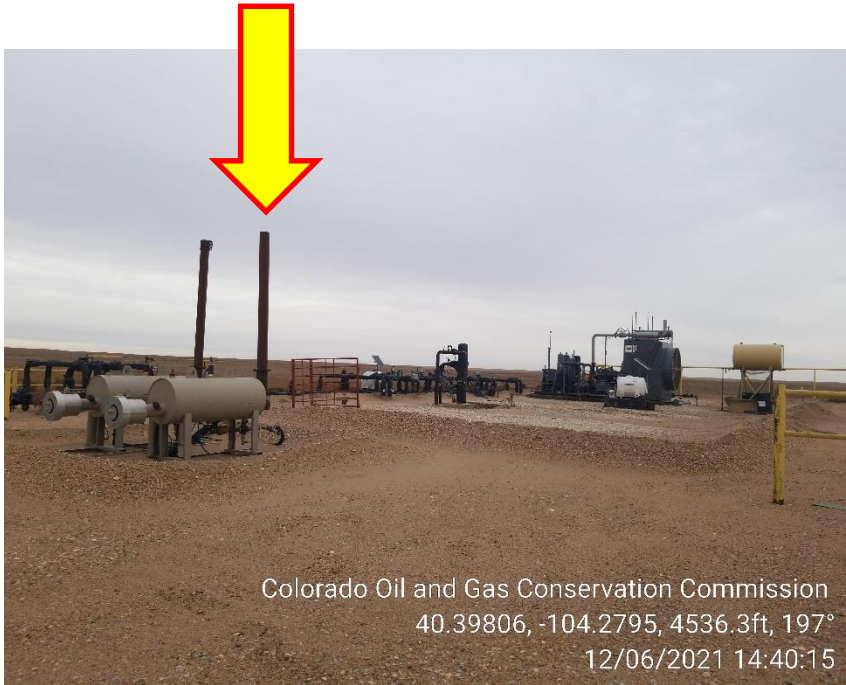
Photo 5 – Glycol Units – South one Missing Wildlife Screen
