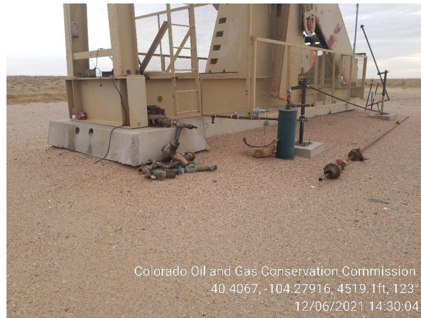
Photo 4 – Unused Wellhead Parts and Polish Rod
