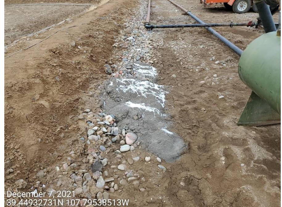
Photo 3: Photos taken from the southeast end of the Location. Photos show grey discolored/impacted soils observed on the fill slopes, and flat areas where the pit previously existed. Photo right shows a pile of grey material (possibly drilling mud) observed on the perimeter of the pad above the slopes in photo 2. Unclear what the observed materials are.
