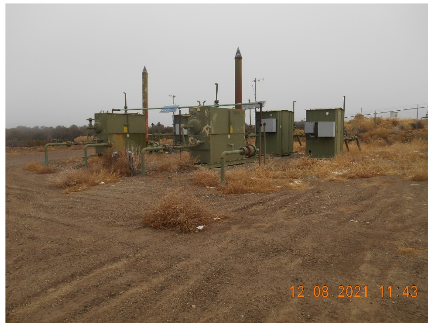
Separator and Meter with sign
