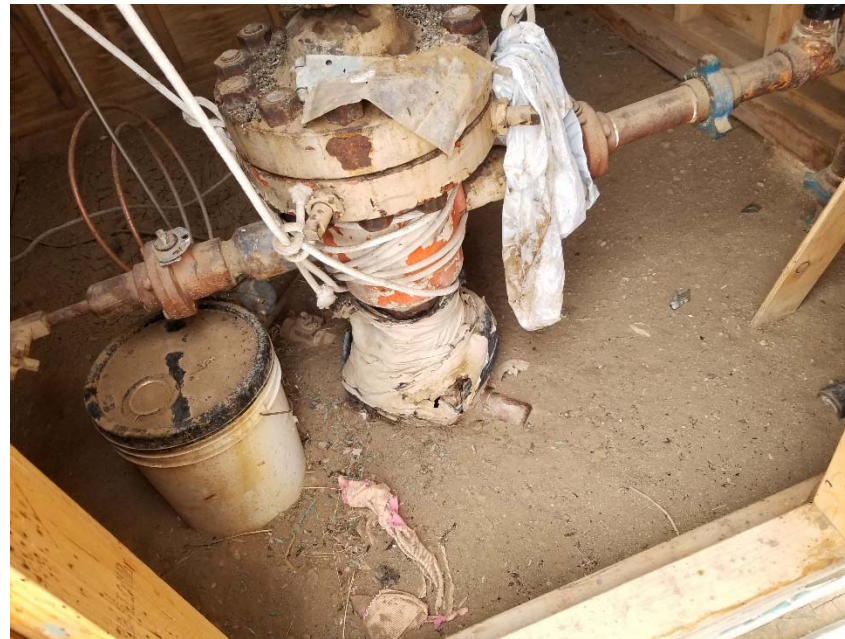
Photo 3. No bradenhead access apparent.
