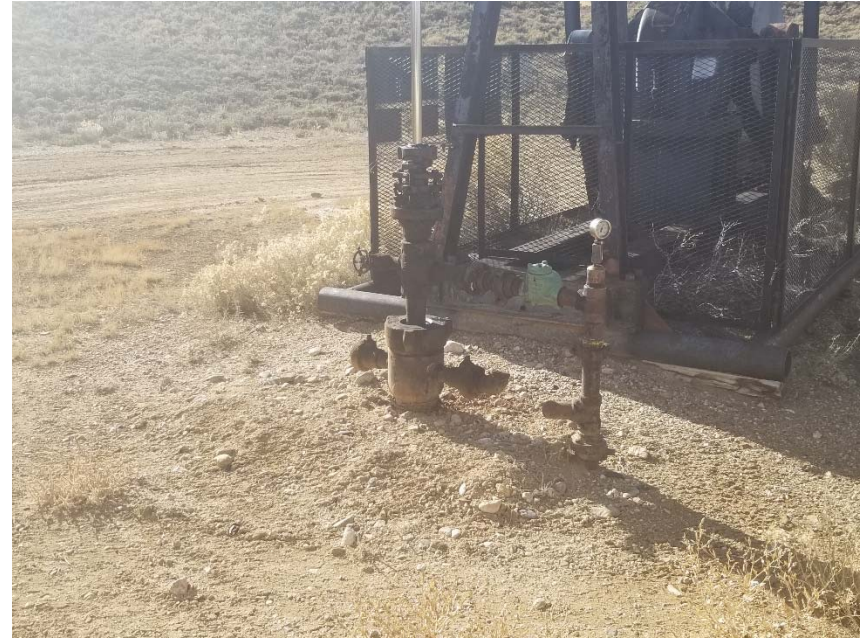
Photo 2. No bradenhead access apparent.
