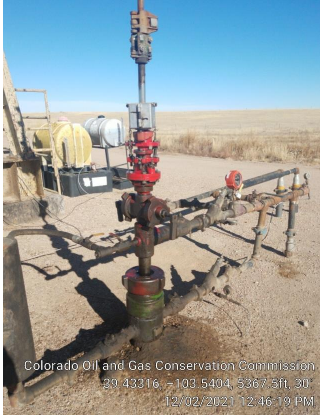
Stuffing Box Leak
