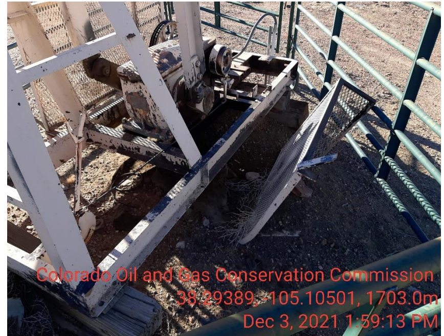
Photo 4 Unused equipment belt guard and stained soil under PU base.
