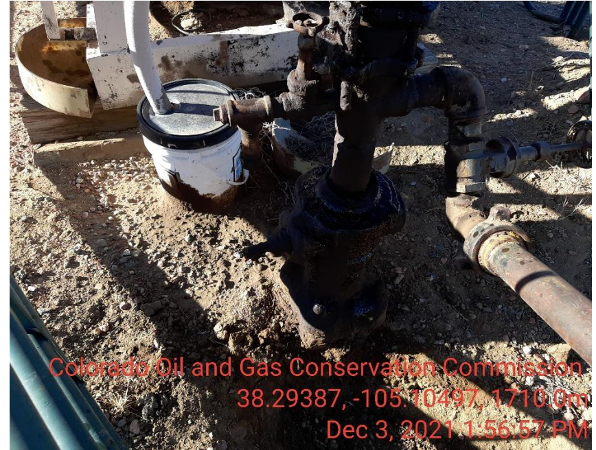
Photo 2 Stained soil around well head and under PU
