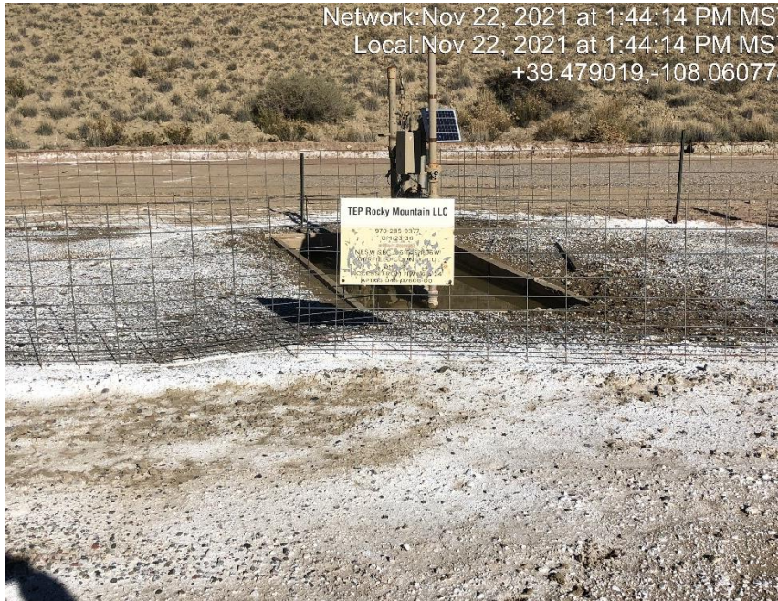
Photo #5224 Wellhead sign weathered and not legible.
