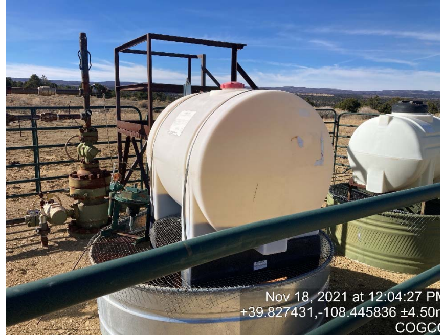
Chemical tank lacking labeling
