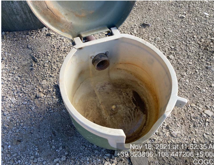
Load line missing caps/bull plugs
