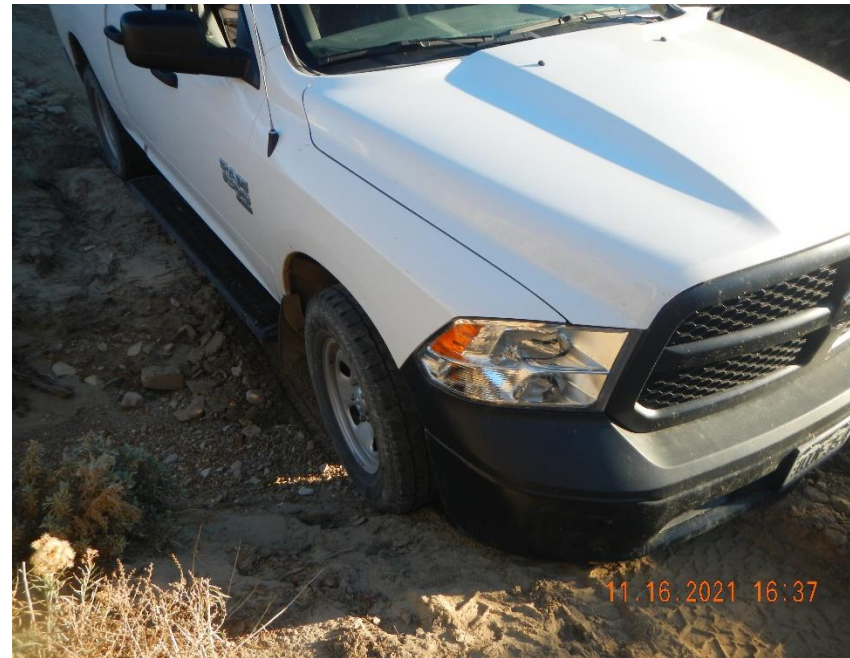
Clearance is poor. Front bumper touching ground passing through low water crossing.
