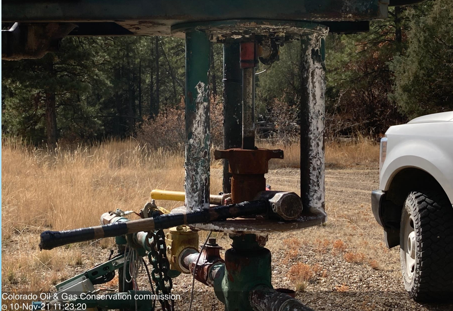
PHOTO 4: CLOSER IMAGE OF WHITE CHALKY BUILDUP ON TR WELLHEAD EQUIPMENT.
