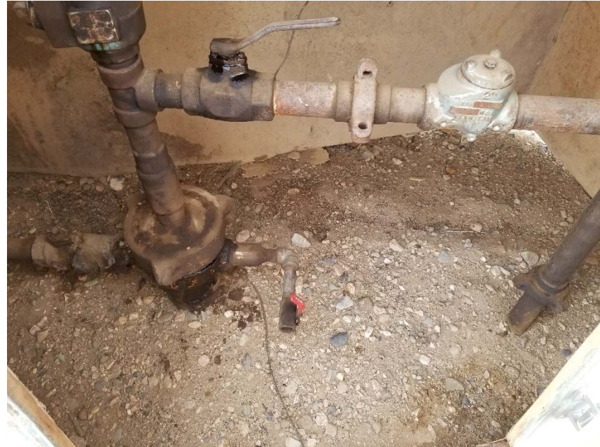
Photo 2. No bradenhead access apparent.
