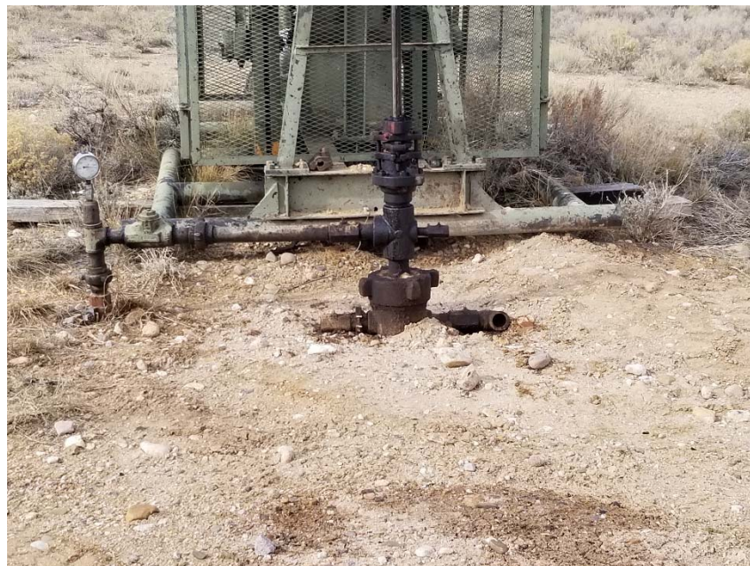
Photo 2. No bradenhead access apparent.
