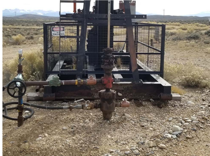
Photo 2. No bradenhead access apparent.
