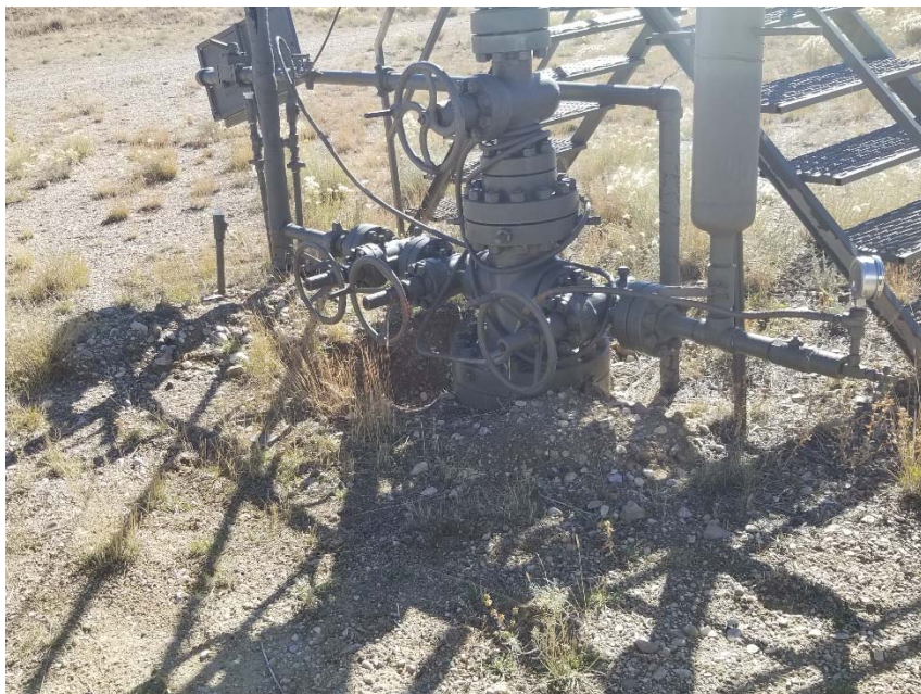
Photo 2. No bradenhead access apparent.
