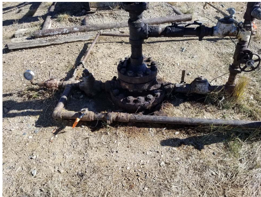
Photo 2. No bradenhead access apparent.
