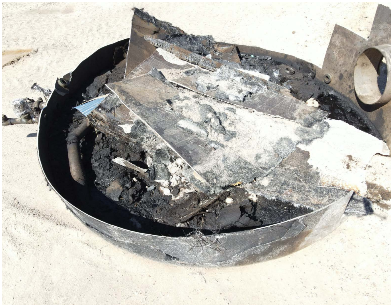
Evidence of a fire found at this tank battery
